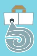
Flush hot water through your drain valve at least once a year to remove sediment build-up
