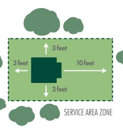
2. Root growth can affect underground power lines Do you have a pad-mount transformer in your yard? That green metal box is a vital part of your electric service and there are highvoltage wires underground leading to the box!
